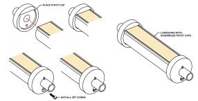
5 Place Pivot Head onto Pivot Cap and secure with blue tape to hold in place. Repeat process for the other end of luminaire.
