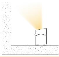
**3** Before installing, place louvers on fixture in sequence to determine positioning and spacing.
