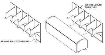
5 Complete the installation by ensuring the louver is consistently aligned across the round shape of the lens.
