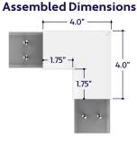
3 Butt fixture extrusions to miter corner, leaving no gaps. Make connections between miter corner and extrusion using included connector plates. Ensure all 4 screws are securely fastened, 2 on each side.
