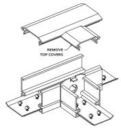
Butt fixture extrusions to miter corner, leaving no gaps. Make connections between miter corner and extrusion using included connector plates. Ensure all 6 screws are securely fastened, 2 on each side.
