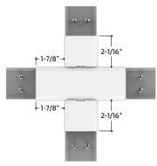
Butt fixture extrusions to miter corner, leaving no gaps. Make connections between miter corner and extrusion using included connector plates.
