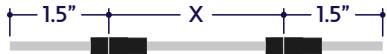
Dry Continuous Connector with White Jacket 20/2 Gauge Wire (A8-CC-2P-DRY-WH-X) X = Specify Length, 3" Default
