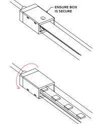
2 Insert the connector box onto the assembled lightstrip and connector, then install the box cap to lock into place.
