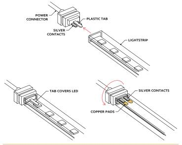
3 Ensure the cap snaps in and is securely fastened, then flip the lightstrip right side up.
