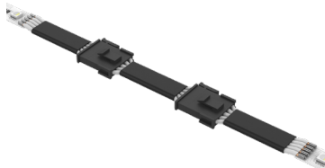
Dry Continuous Connector with Black Jacket (20/5 Gauge Wire) (A8-ZIZA-TAPE-CC-DRY-BK-X) X = Specify Length, 3" Default
