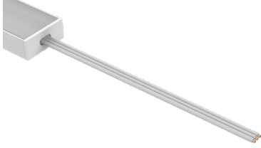
Dry Power Connector (20/3 Gauge Wire) (A8-ZOMU-SDL-PC-DRY-X) X = Specify Length, 36" Default, 25' Maximum
